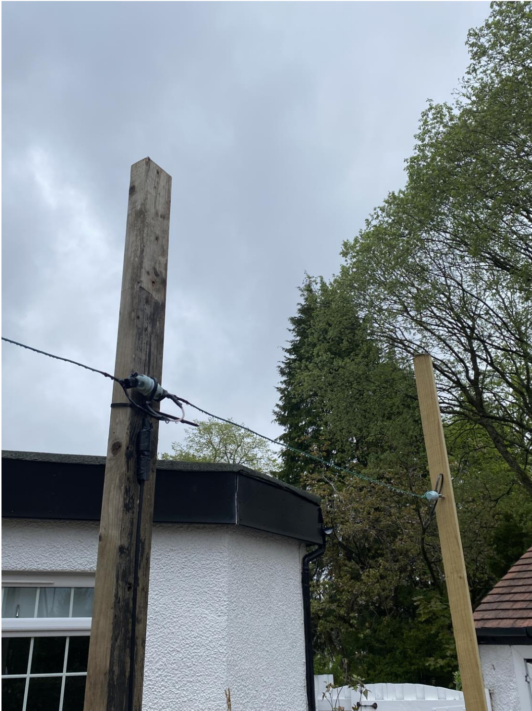
Fig. 7: Half wavelength simple dipole to observe solar radio bursts around 64-72 MHz
