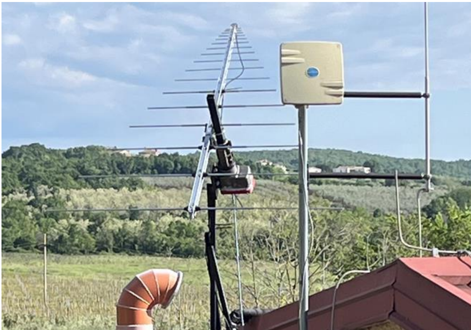
Fig. 1: LPDA CLP-5130 with Sun-tracker
