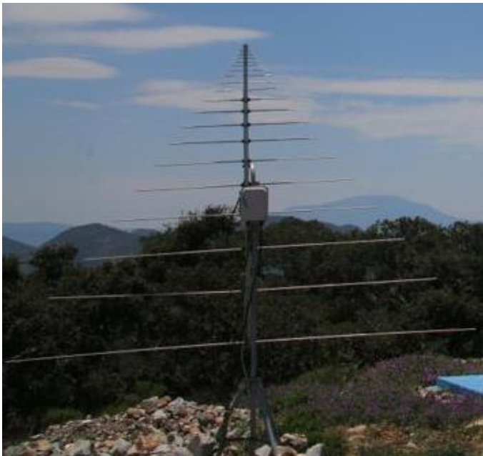
Fig. 1: Left: LPDA and frontend (LNA) Right: 1 st light with start frequency of a type II burst
