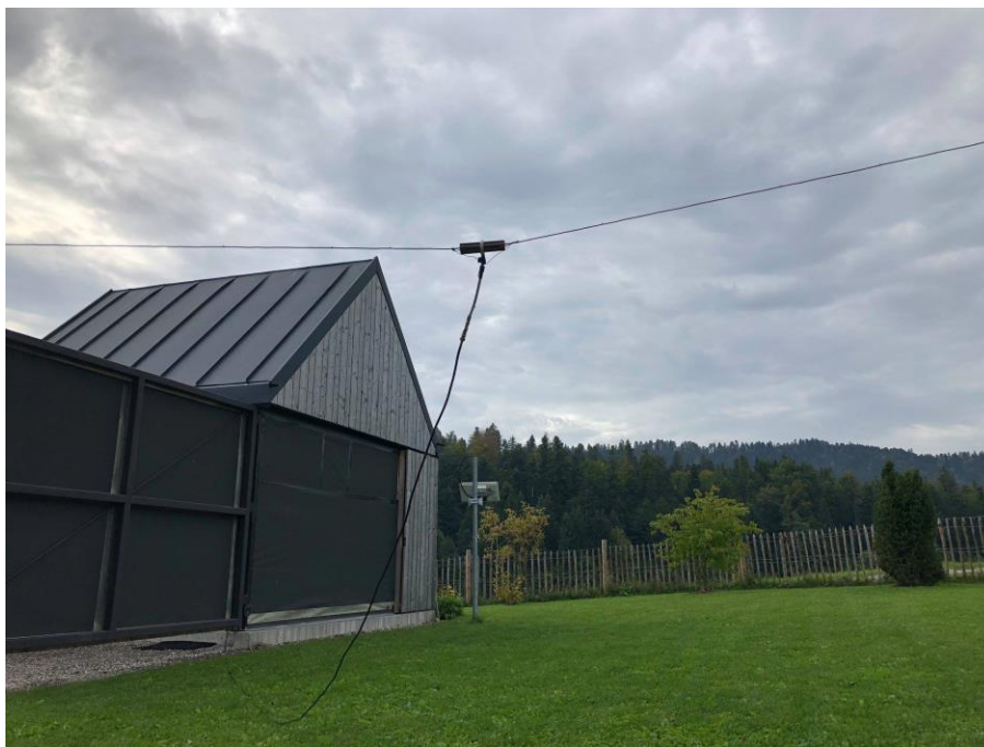
Fig. 4: Simple dipole to observe low frequency radiation from the Sun, taken from Facebook (Fritz&Paul)
