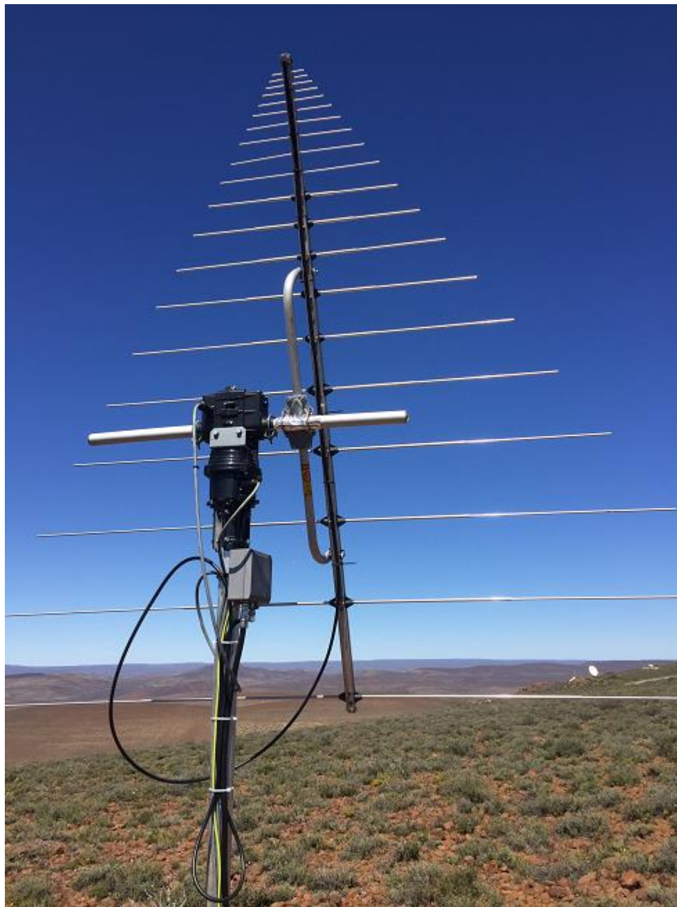
Fig. 2: Close up of LPDA, positioning system and frontend containing low noise amplifier.
