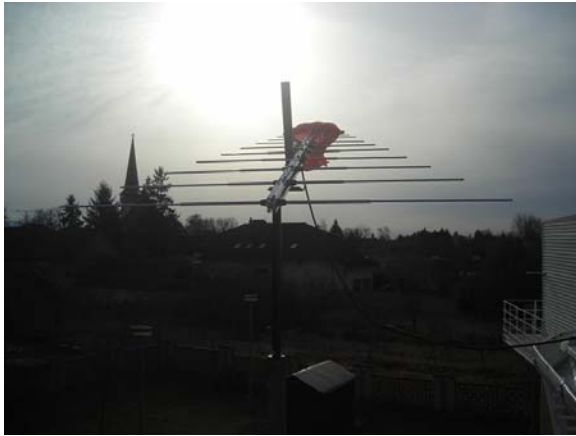
Fig. 1: Left: Logarithmic-periodic antenna from CREATE covering 50 MHz – 1300 MHz, see also: http://www.grove-ent.com/ANT16.html
