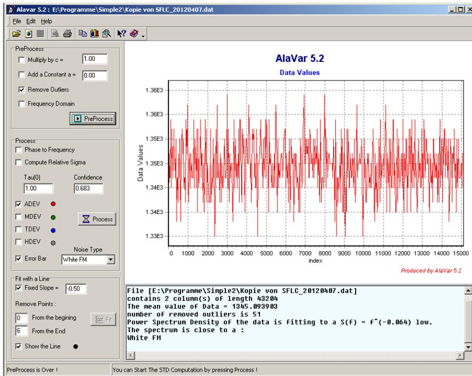
Figure 3: PreProcess of sampled data at one single frequency channel and generating light curve. The plot shows noise with rather low interference (no large spikes or gaps). The x-axis shows the sample number and the y-axis the measured voltage in millivolts.
