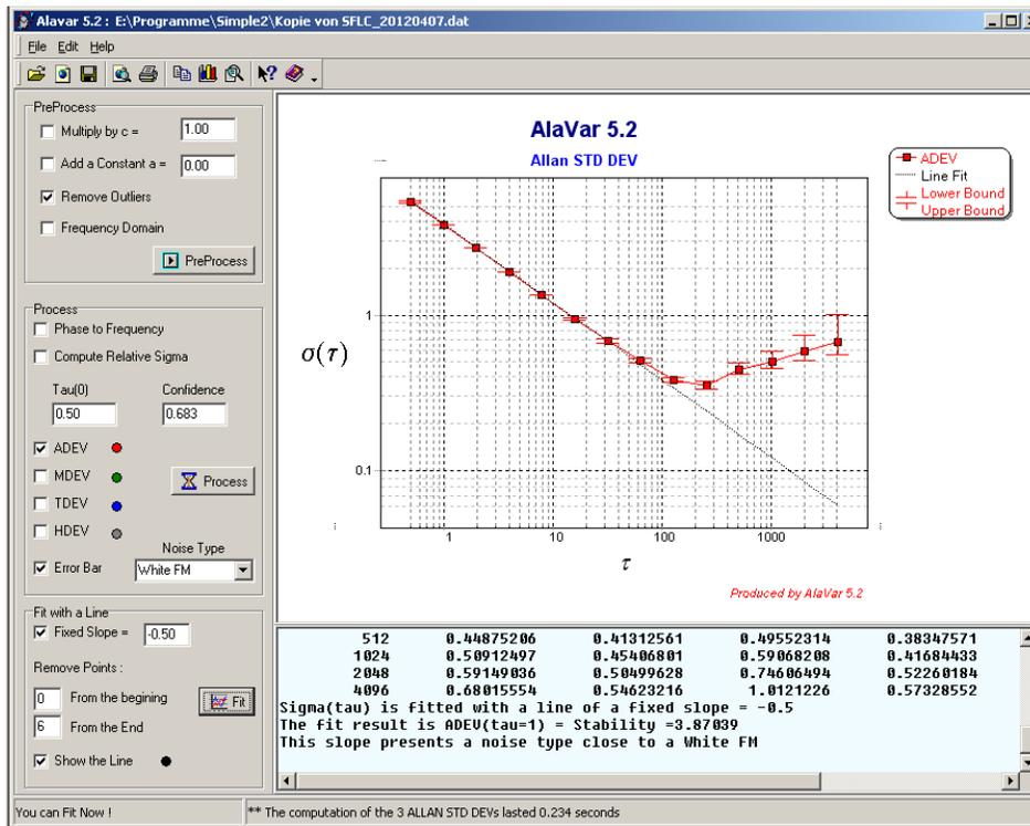
Figure 4: ALLAN-variance plot for Callisto at  $f = 610.0 \text{ MHz}$ . The x-axis shows the integration time  $\tau$  expressed in seconds over an observation time of 6 hours and 3 minutes, the y-axis the variance  $\sigma$  of the signal, both in logarithmic scale.
