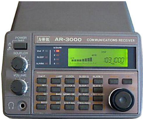
Fig. 4 ~ Communication receiver AR-3000A, controlled via RS-232 from a standard PC.
