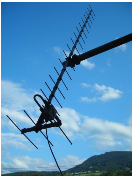
Fig. 3 ~ 610 MHz Yagi on the balcony, pointing to the meridian position of the Sun.
