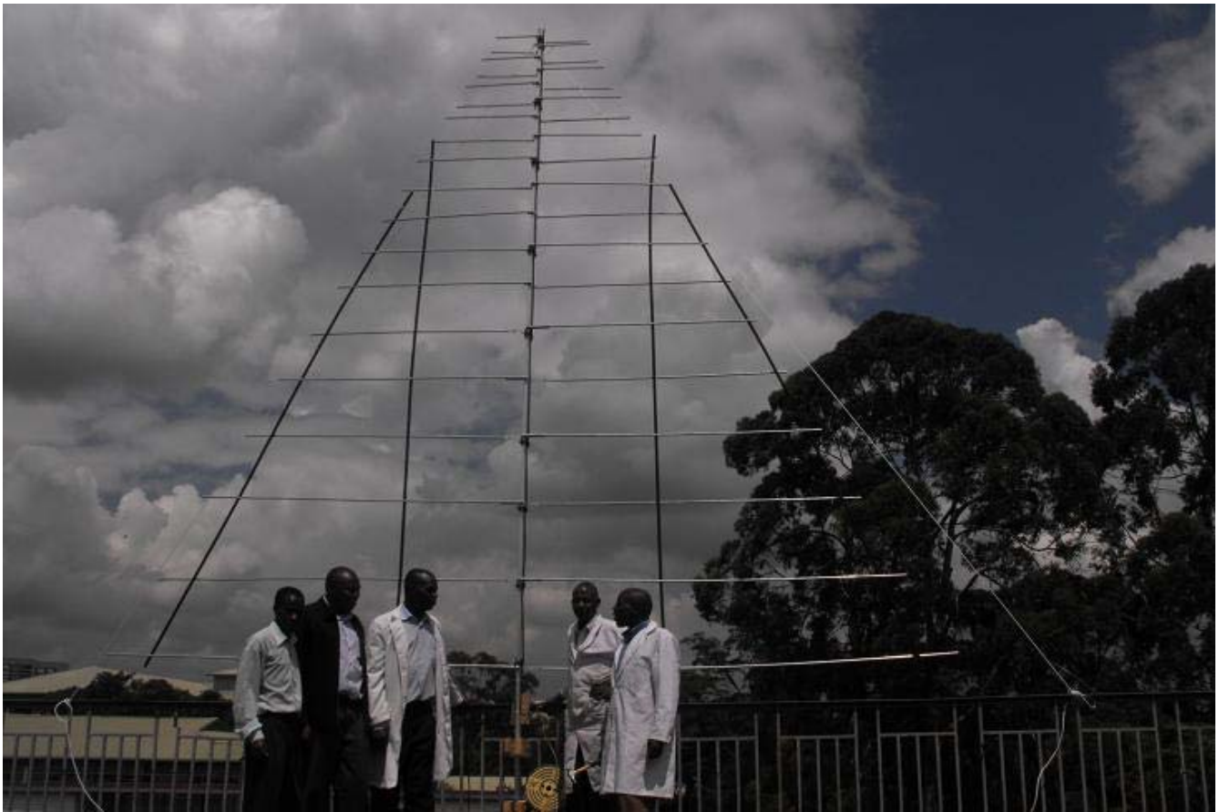
Fig. 1: Low frequency logarithmic-periodic antenna covering about 20 MHz – 160 MHz pointing to zenith. The antenna was built in the mechanical workshop of UoN with aluminum profiles from local stores. Preamplifier and Callisto are directly underneath the antenna in one of the offices of UoN.
