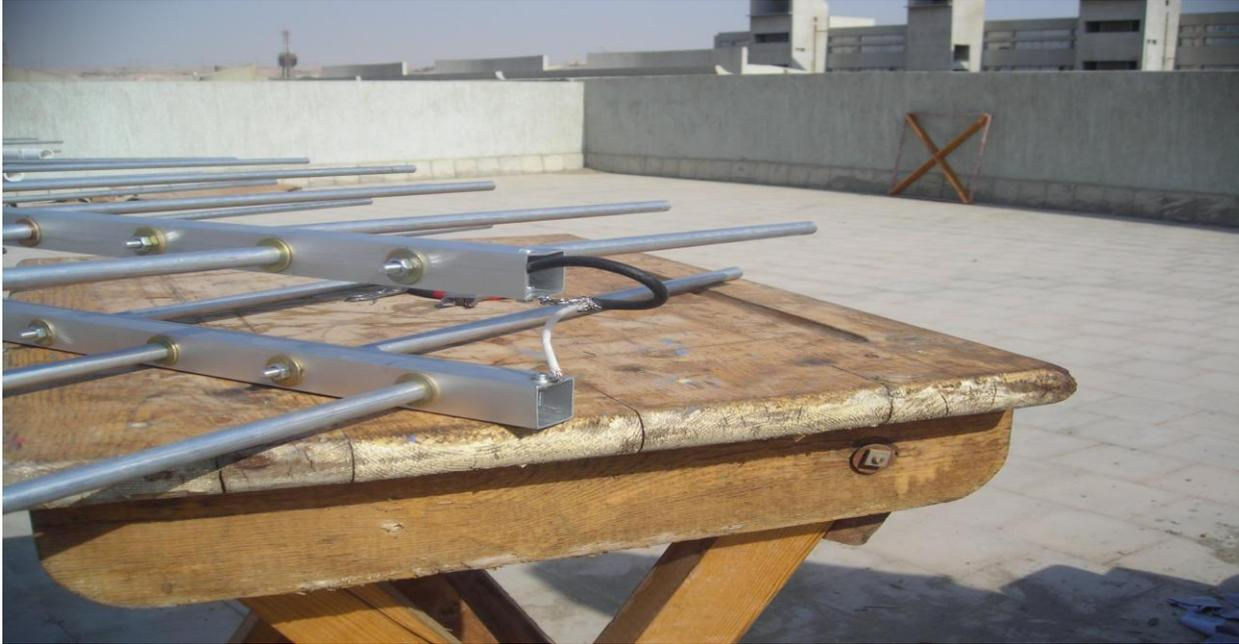
*We should connect the the wires inside each boom in order not destroy form sun and weather conditions.*
