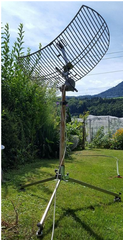
Fig. 7: S-band antenna with a satellite rotor on a tripod tracking the Sun
