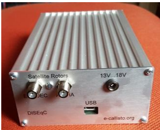
Fig. 1: Back panel of the DiSEqC tracker with two F-connectors for satellite rotors, USB-control port and DC-input
