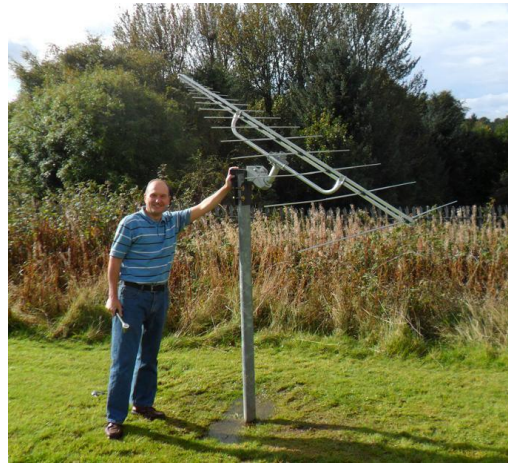
Fig. 6: How to install SAT-rotor for pseudo parallactic mount with tracking in local hour angle only at fixed declination. Declination is changed manually 2...4 times a year.
