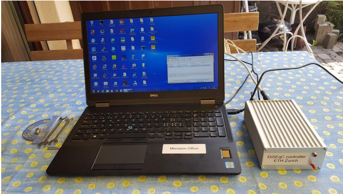
Fig. 9: Control notebook with Windows 7 and the rotor controller box. A Python script is called every 5 minutes by the Splinterware System Scheduler program (ssfrees.exe) and is commanding the rotor in figure 7 to the actual Sun position.
