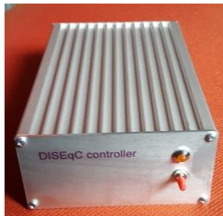
Fig. 2: Front panel with power switch and LED
