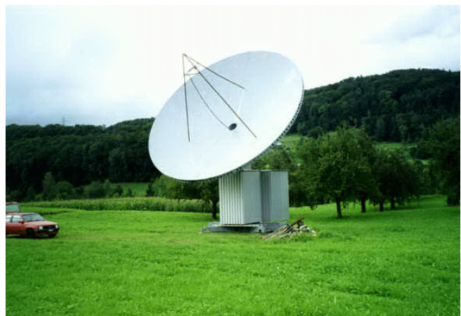
Fig.1. View from South-East to the semi professional radio telescope with a 10m full metal parabola antenna near Ermenswil Switzerland. The shack with the radio frequency electronics is shielded by an additional metal cabinet against electro magnetic disturbances.
