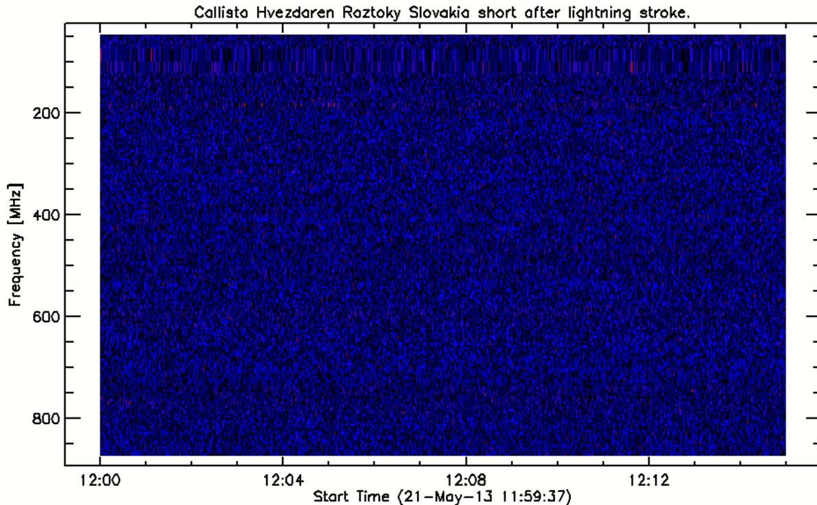
Figure 2: Spectrum after lightning strokes damaged the preamplifier, a Mini-Circuits low noise amplifier. The amplifier no longer provides amplification, and we only see receiver noise and no signature of any local RFI from nearby transmitters. One might get the impression the installation is in a radio quiet area with no RFI but this is obviously wrong.
