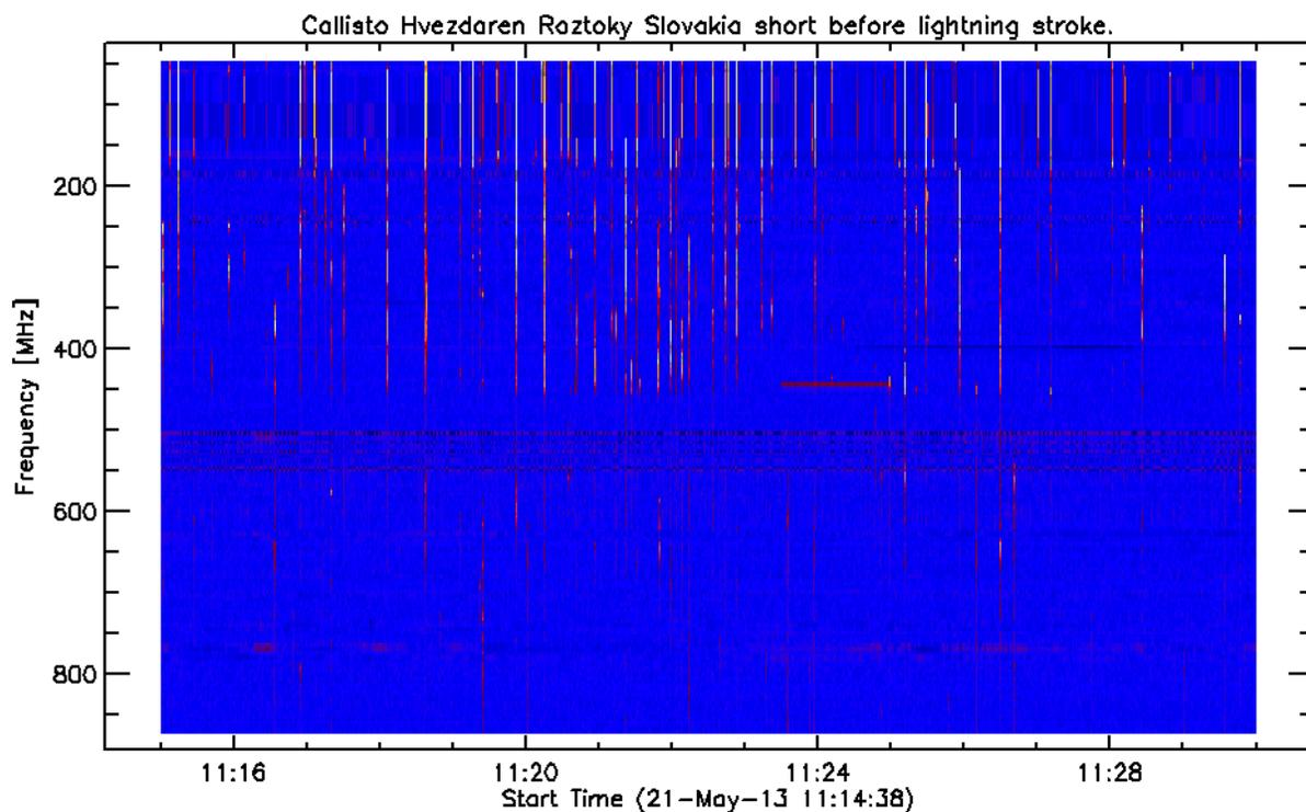
Figure 1: Radio spectrum with large amount of individual lightning strokes (bright vertical structures). Horizontal structures are due to local RFI (broadcast television-transmitters). Blue color denotes to background noise of the receiver and sky.
