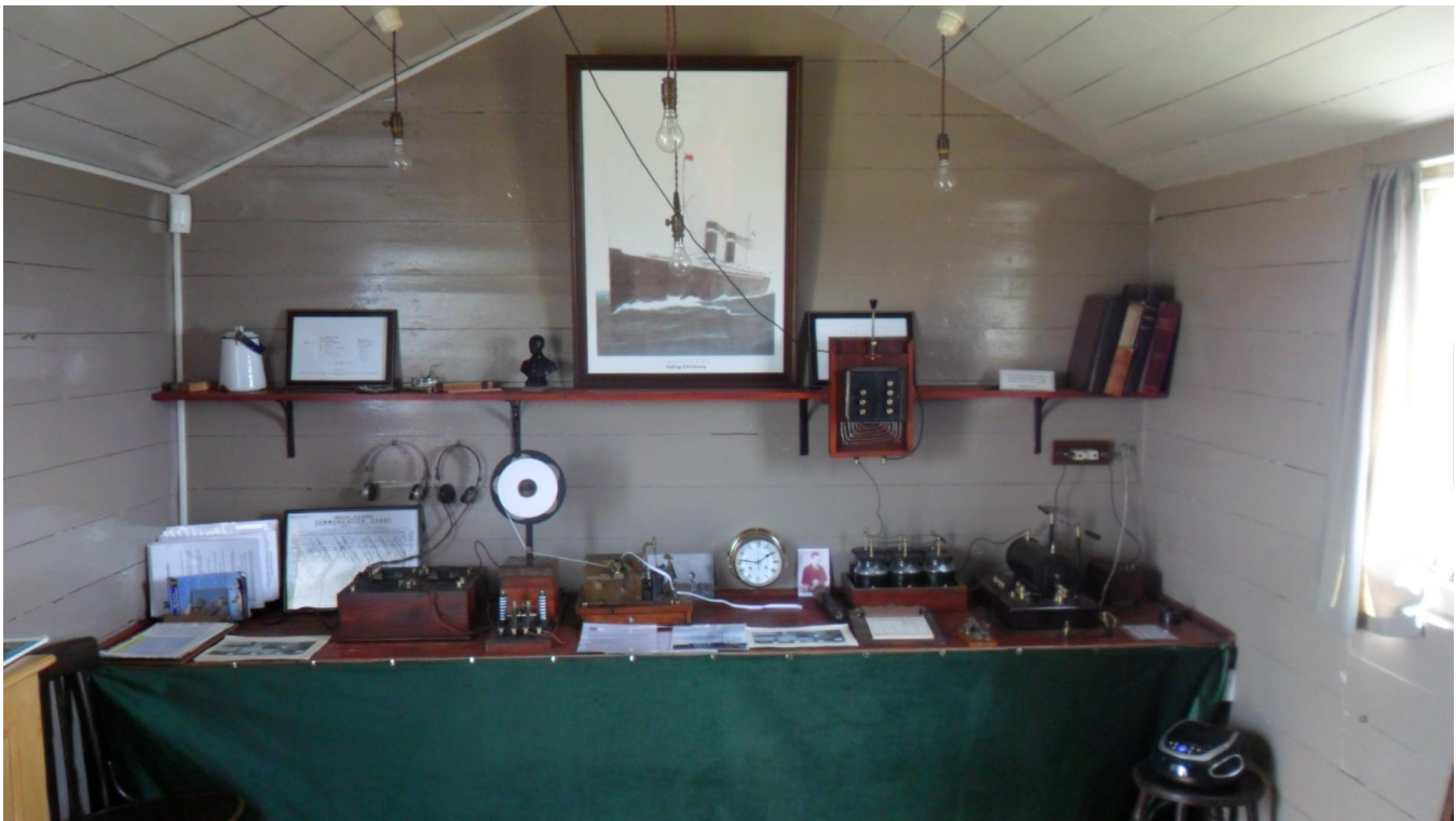
Figure 2 ~ Receiver with Morse code puncher on the left side, Leyden jars (a type of battery) with induction coil, spark gap and Morse key on the right side.
