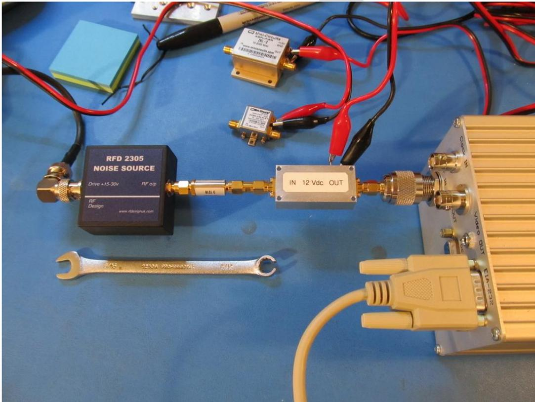
Figure aa ~ Noise figure measurement setup for the CxLNA. Other amplifiers used the same setup. The RFD2305 noise source (blue box on left) was connected directly to the RF Input of the amplifier. The RFD2305 includes a 10 dB attenuator and has ENR = 5.8 dB. The amplifiers were connected to a power supply using temporary leads (middle). The Callisto (right) was setup in the normal way with EIA-232 connection to the PC and power connection to a 12 Vdc power supply.
