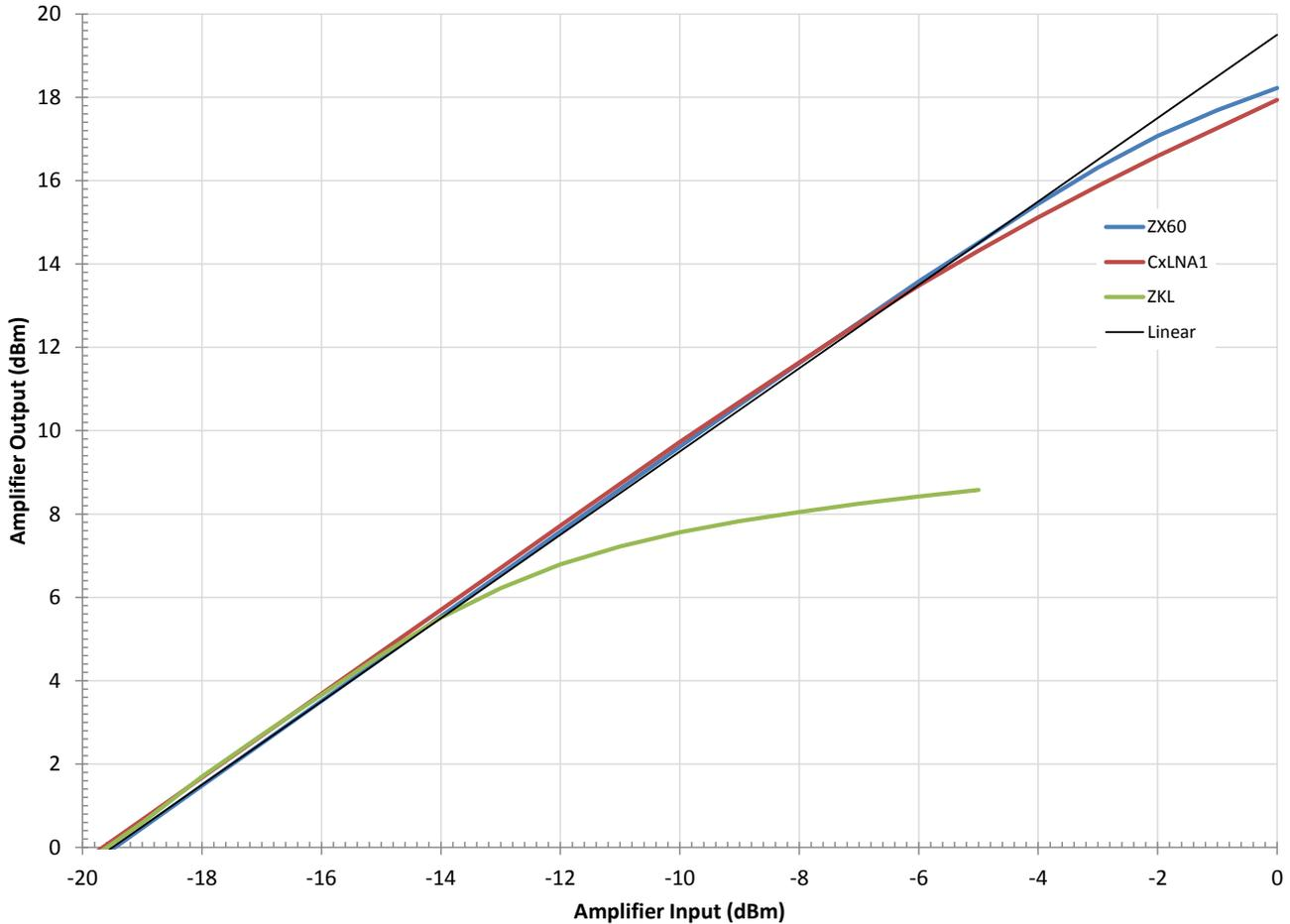
Figure 4 ~ Overload compression for the three amplifiers. A usual measure is the 1 dB compression point, where the linearity of the amplifier changes by 1 dB. The ZX60 and CxLNA have nearly identical performance at high input powers, with the compression point approximately  $-3$  dBm. The higher gain ZKL amplifier has a much lower compression point at approximately  $-12$  dBm.
