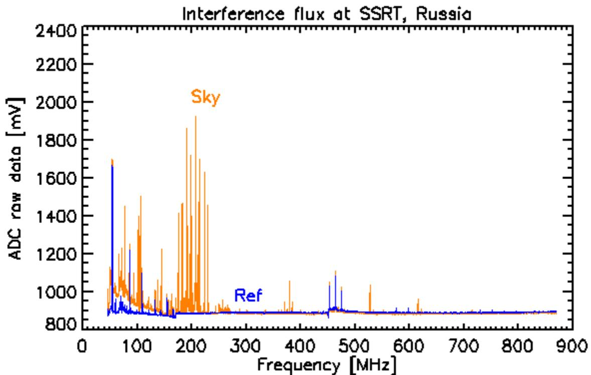
Figure 1b: Raw data of the spectral overview as captured by Callisto in Siberia. Orange plot denotes to data while observing the sky and blue plot denotes to the observation of a 50  $\Omega$  resistor. Y-axis shows measured voltages of the ADC expressed in mV versus the observed frequency in MHz. Badary in Siberia is suffering from only low level interference around 200 MHz.
