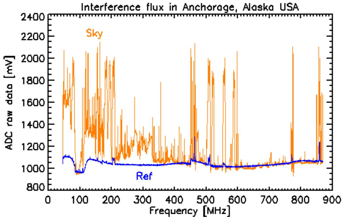
Figure 1a: Raw data of the spectral overview as captured by Callisto in Alaska. Orange plot denotes to data while observing the sky and blue plot denotes to the observation of a 50  $\Omega$  resistor. Y-axis shows measured voltages of the ADC expressed in mV versus the observed frequency in MHz. Anchorage is suffering from a lot of high level interference. Near 100 MHz the whole FM-range is suppressed ed with a notch-filter.
