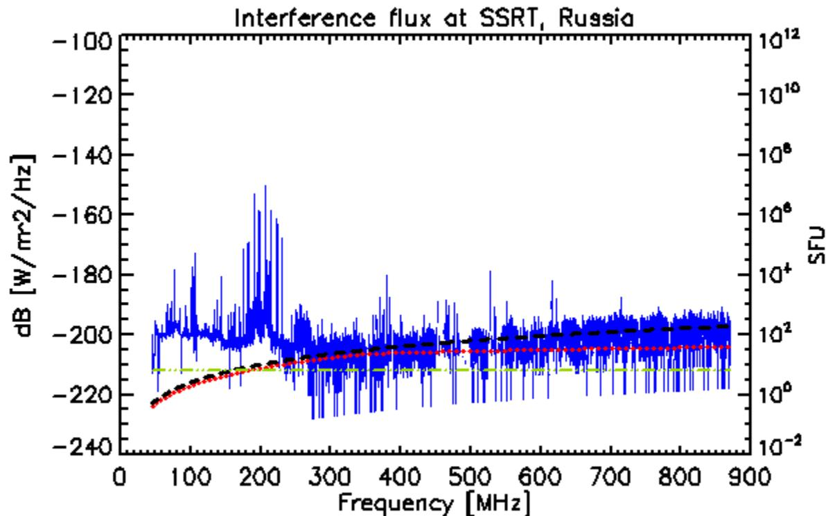
Figure 3b: Measured sensitivity of the instrument in Badary/Siberia (blue solid line), quiet solar flux (red dotted line), calculated instrumental sensitivity assuming no interference (black dashed line) and upper limit for VLBI observations at 325.3 MHz (green dashed/dotted line). Many frequencies above 300 MHz can be used to detected quiet solar radio flux in Siberia under the current conditions. Near 240 MHz we can detect transponders signals from military satellites.
