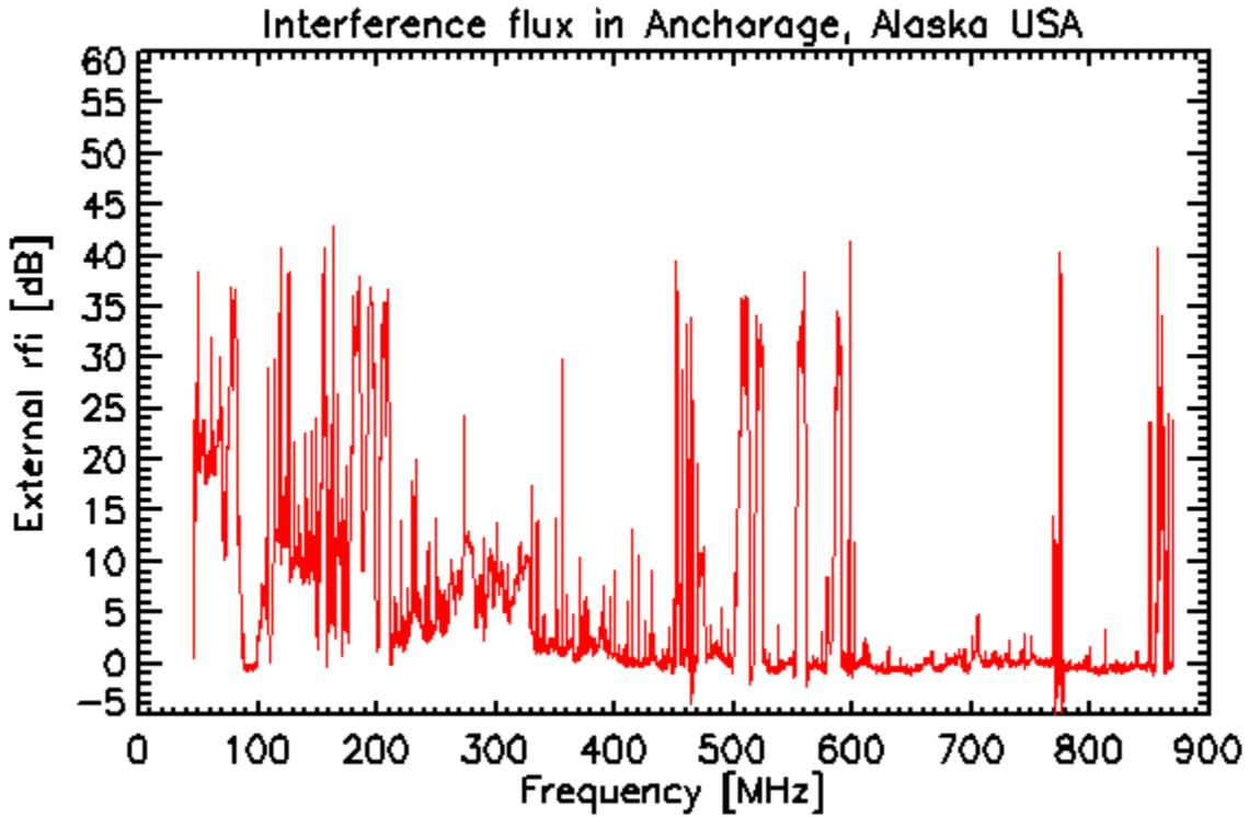
Figure 2a: Difference plot ( $V_{\text{Sky}} - V_{\text{Ref}}$ ) from Anchorage expressed in dB versus frequency in MHz. This plot is named as external rfi because the internal noise and interference is subtracted from the sky-measurement.
