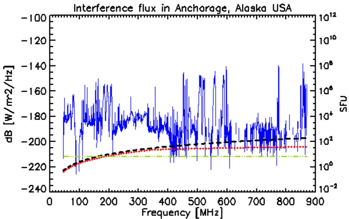
Figure 3a: Measured sensitivity of the instrument in Anchorage (blue solid line), quiet solar flux (red dotted line), calculated instrumental sensitivity assuming no interference (black dashed line) and upper limit for VLBI observations at 325.3 MHz (green dashed/dotted line). Only a very few frequencies near 400 MHz and between 600 MHz and 750 MHz can be used to detected quiet solar radio flux in Anchorage under the current conditions.
