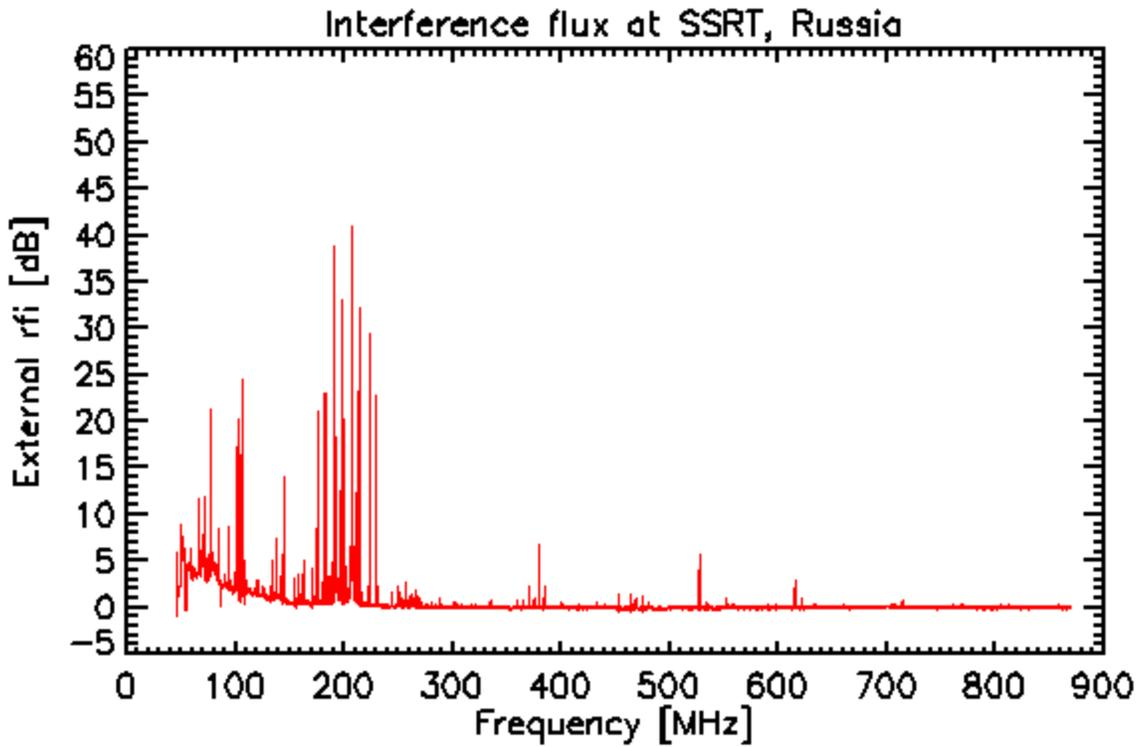
Figure 2b: Difference plot ( $V_{\text{Sky}} - V_{\text{Ref}}$ ) from Siberia expressed in dB versus frequency in MHz. This plot is named as external rfi because the internal noise and interference is subtracted from the sky-measurement.
