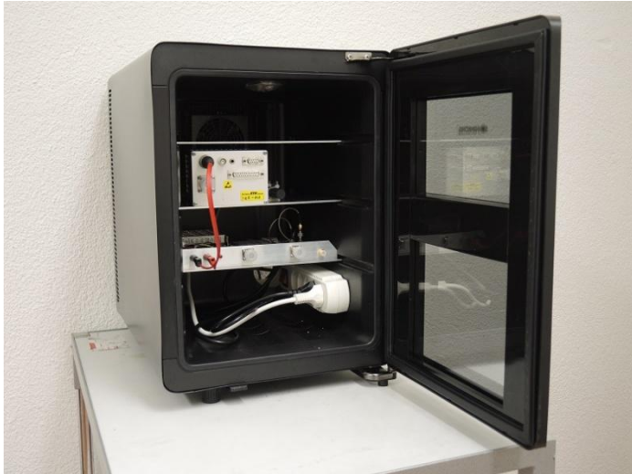
Figure 3~ This commercial wine cooler contains from bottom to top: Power distribution 230 Vac, heterodyne receiver 960 MHz ... 1260 MHz down to UHF-range 750 MHz ... 450 MHz, Callisto spectrometer [Benz (2004)] and a separate temperature-humidity sensor. This wine cooler is based on a Peltier-cooling system in the backplane and a control panel embedded in the front door. Temperature range can be set digitally between 12°C and 18°C. All coaxial- and control (RS-232) cables are fed through a hole in the backplane which was closed after installation by Urethane foam.
