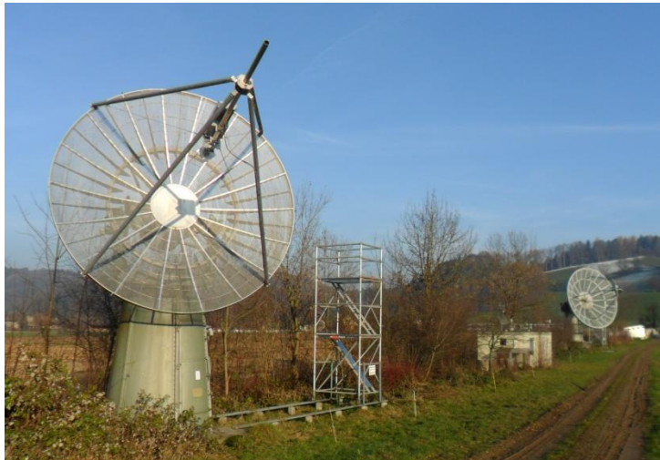
Figure 1~ 5 m parabolic dish (left) at Bleien with a linear polarized LPDA in the focal plane. A 7 m parabolic dish for solar observations can be seen in the background at right.
