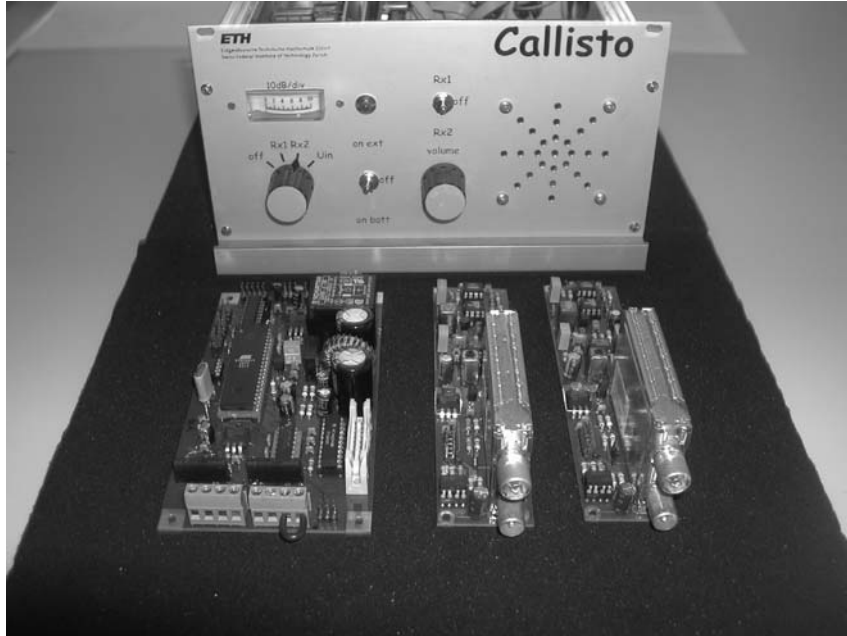
Figure 2. The hardware of CALLISTO shown in the foreground consists of the main board for data acquisition and interface with a RISC processor ATmega16 (left) and of two synchronous receivers (right). The complete spectrometer is shown in the background. Its physical size (width) is 24 cm.
