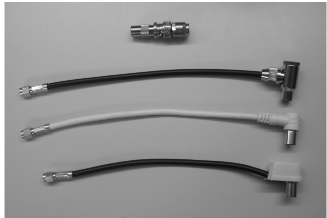
Fig. 1. From top to bottom: - Termination 50Ω as reference, - ideal cable RG-58 (black) with shielded connector from Conrad (metal), - commercial cable 75Ω (white) with unknown angle connector (white), - RG-58 (black) with low cost angle connector from Pusterla (white).
